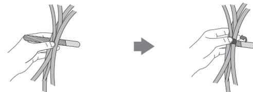
Fasten the cables with the cable tie
