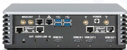
Cynap connectors with HDBaseT option
