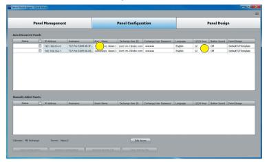
Click on the Panel Configuration tab. Each panel IP Address and Hostname are shown. The Language, Clock Format, Button Sound and Panel Design are set to default values that can be changed.
