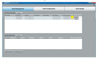
Each panel requires setup. Click on the first panel's Setup button which will connect to the device.
