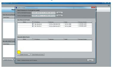
When firmware has been selected for a panel model and checkbox has been selected, the Update Firmware button becomes enabled.
