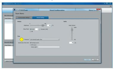
The General Setting tab allows the panel hardware settings, including brightness, sleep mode, and audio levels, to be changed. The timezone and clock synchronization can also be set within this tab.
