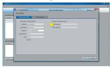
The Communication Settings tab is displayed under the Device Management Window. Confirm that the panel is correctly configured. It is highly-recommended that you change the password for the panel.
