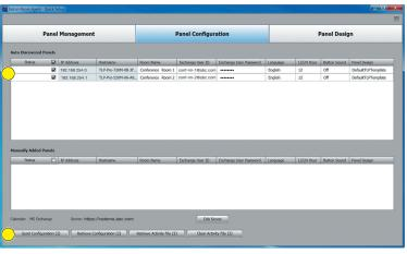
When all the required entries for a touchpanel have been completed and the checkbox has been selected, the Send Configuration button becomes enabled.
