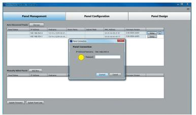
The Panel Connection dialog box is displayed. The default password on panels shipped from Extron is "extron" - case-sensitive.
